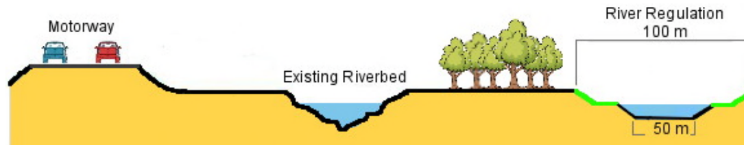
Figure 3-7. Typical Cross-Section of the Regulated Channel
